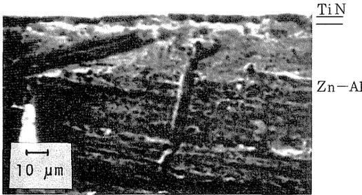
Fig. 3 SEM images of the section of TiN film ion-plated onto a Zn-Al substrate.
