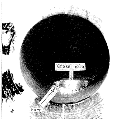
Fig. 2 Burrs generated inside main hole before ball burnishing.
