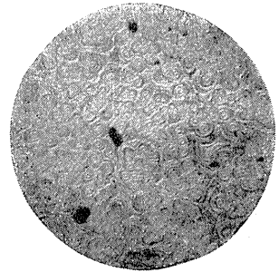
Phot. 3. The annual-ring like stru- cture of Se-plate, in the 1st stage of treatment. \times 333
