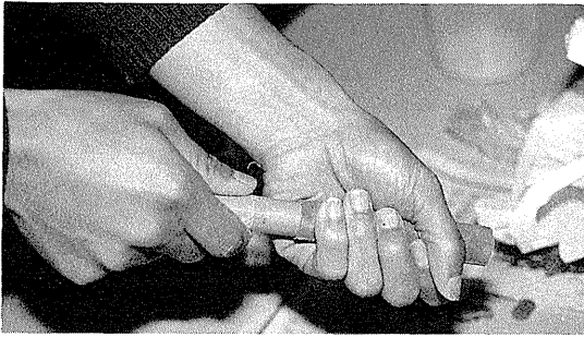
Photo. 14 Removing Cement Mortar Specimen from the mold: Step 3 The mandrel is removed by the same method as in Photo. 7
