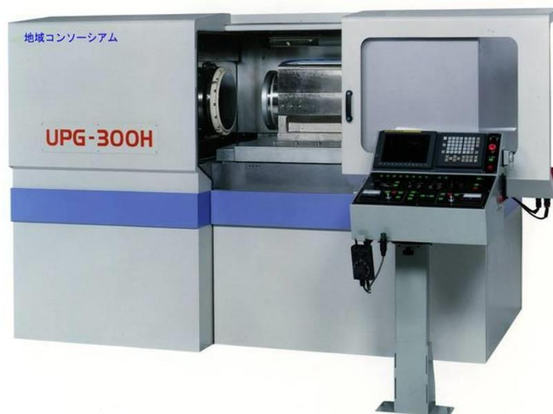
Fig. 2.9 The configuration of wafer grinding machining tool
